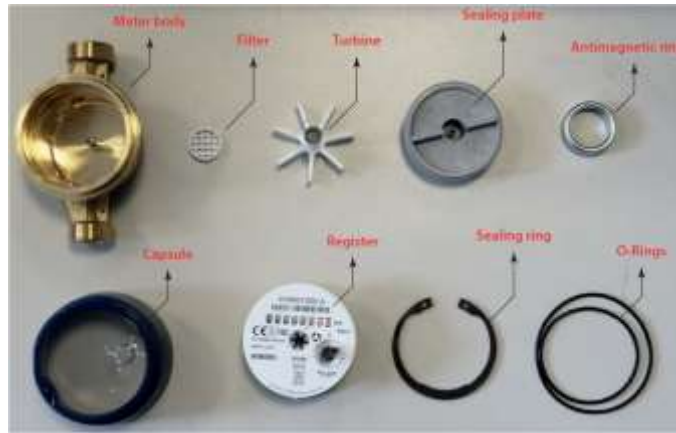
Illustration 3 Photograph showing water meter components.
