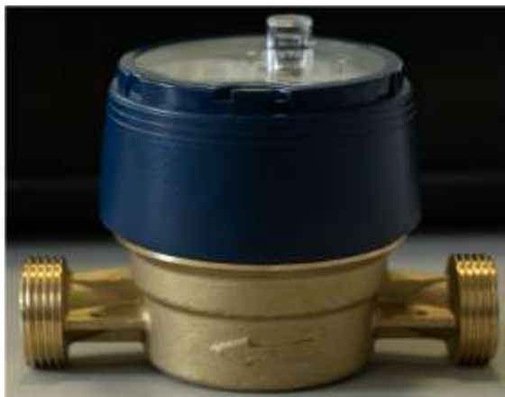
Illustration 1 Photograph showing the water meter.
